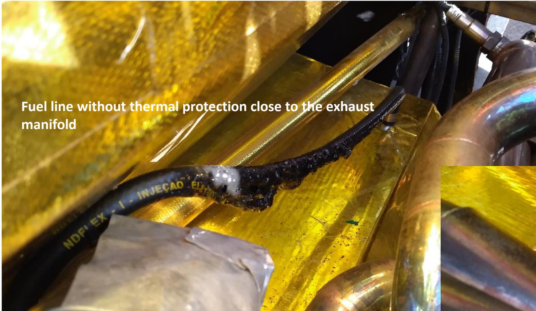
The team set up the fuel line with protection and a new route, with a safe distance from the exhaust manifold.
