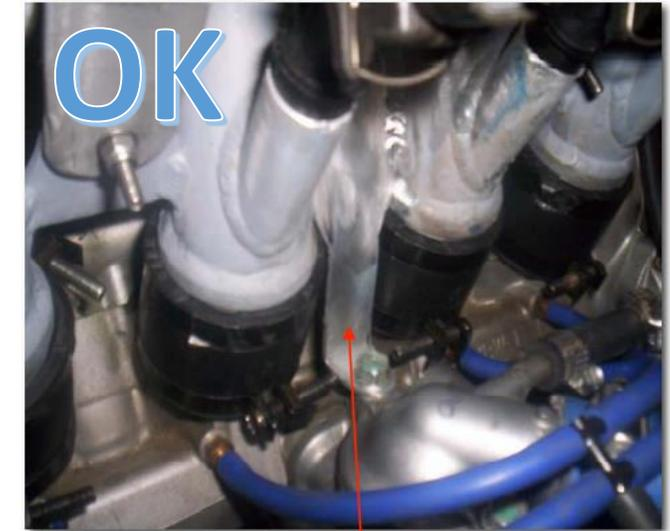
Intake Manifold – The intake manifold must be securely attached to the engine block or cylinder head with brackets and mechanical fasteners. This precludes the use of hose clamps, plastic ties, or safety wires. The use of rubber bushings or hose is acceptable for creating and sealing air passages, but is not considered a structural attachment.
