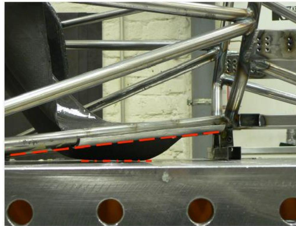
The lowest point of the driver's seat must be no lower than the bottom surface of the lower frame rails or by having a longitudinal tube (or tubes) that meets the requirements for Side Impact tubing, passing underneath the lowest point of the seat.
