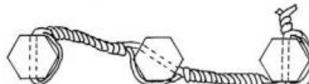
DOUBLE TWIST METHOD - MULTIPLE FASTENER
